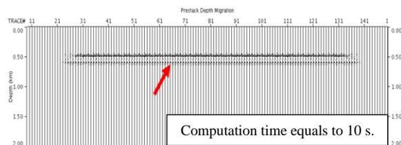
Figure 5: The imaging result of the correlation window with 9 traces. The red arrow indicates the artificial noise.
