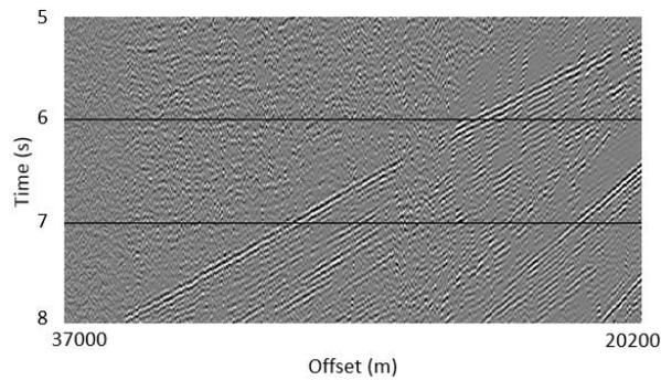
Figure 12: The enhanced refraction after applying the super-virtual interferometry.
