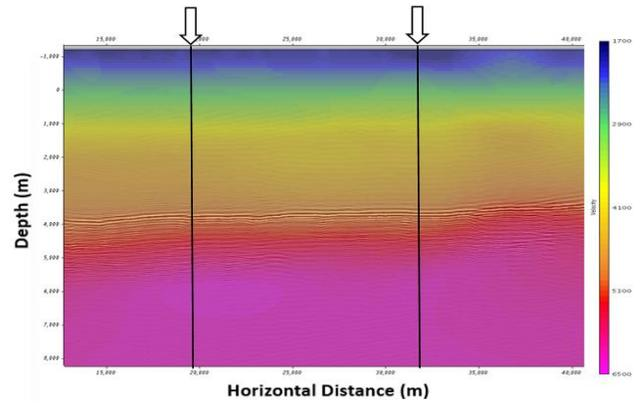
Figure 14: The overlaid model and migration image. The black lines indicate the CMP locations of Figure 11.
