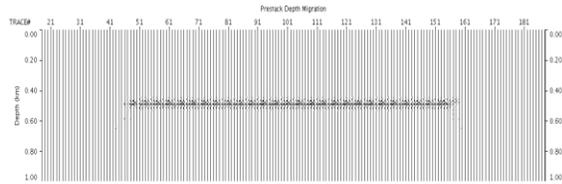
Figure 6: The original imaging result of the refraction migration.
