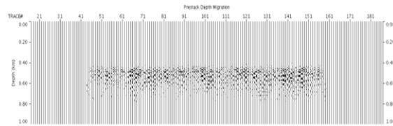
Figure 8: The imaging result when the SNR of refraction equals to 1.
