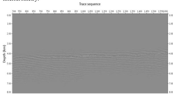
Figure 13: The prestack depth migration result of the real dataset.
