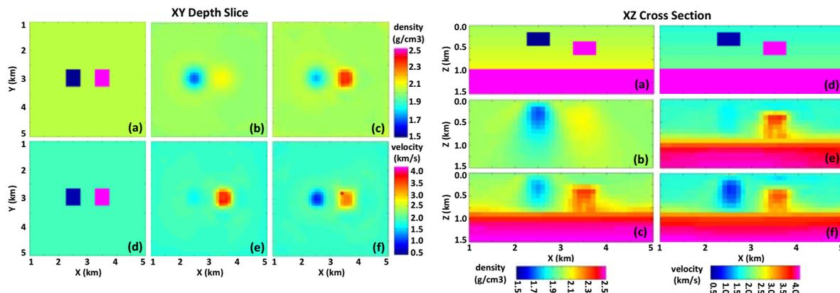
**Figure 1:** Comparison of density and velocity models along an XY depth slice at 400 m and an XZ cross section through the center of the model. The results as single domain inversions and as multi domain joint inversion are shown in (a) synthetic density model, (b) density from single domain inversion, (c) density from joint inversion, (d) synthetic velocity model, (e) velocity from travel time inversion and (f) velocity reconstruction from joint inversion.
