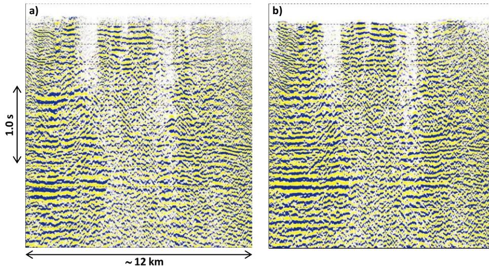
**Figure 2:** Stack with (a) elevation statics correction; and (b) wave-equation datuming using the near-surface velocity model derived from the joint inversion of seismic and gravity data.
