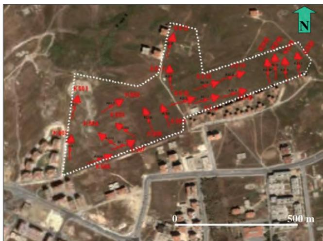
**Figure 8.** Location map for the seismic survey within a residential development project site in Istanbul. The survey consists of refraction profiling at 20 locations. The arrows represent the receiver spread directions at each location.
