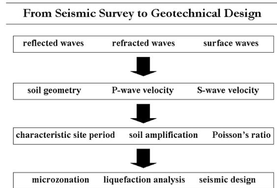
Specifically, the layer thicknesses and S-wave velocities within the soil column are used to compute the characteristic site period. The response spectrum computed from the near-surface model is used to estimate the amplification factor for the soil column. The P- and S-wave velocities associated with the near-surface are used to compute a Poisson's ratio profile in depth. Finally, assuming an empirical relation between density and P-wave
