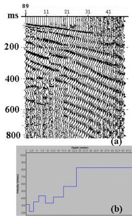
Figure 3. (a) A field record that exhibits a dispersive wave package associated with Rayleigh waves, and (b) the S-wave velocity profile in depth derived from the Rayleigh waves in (a) using an inversion procedure (Table 4).
