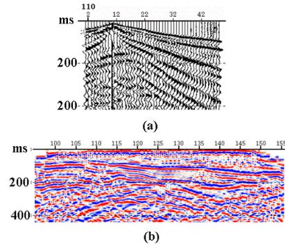
Figure 1. (a) A field record with a good reflection at 200 ms, and (b) the CMP stack derived from 75 shot records as in (a) using a simple processing sequence (Table 2).
