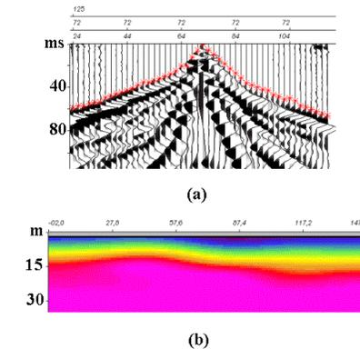
Figure 2. (a) A field record with picked first breaks, and (b) the P-wave velocity-depth model derived from refracted arrivals as in (a) using a traveltimes inversion procedure (Table 3).
