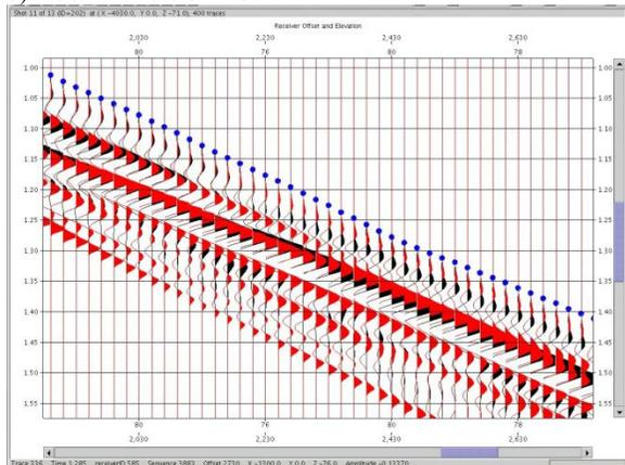
Figure 4: a) synthetics (red) and input data (black) after 9 iterations from waveform inversion; b) synthetics (red) and input data (black) after 9 iterations from joint inversion.
