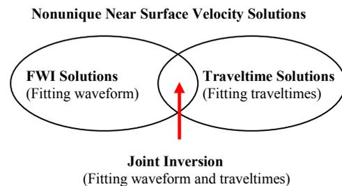
Figure 1: Schematic plot explaining the idea of joint inversion for constraining nonunique near surface velocity solutions.
