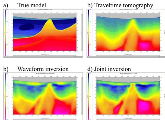
Figure 2: Synthetic experiment: a) true model; b) traveltime tomography result; c) waveform inversion result; d) joint traveltime and waveform inversion.
