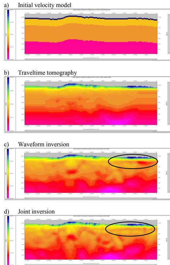
Figure 3: a) Initial velocity model; b) traveltime tomography solution; c) waveform inversion solution; d) joint traveltime and waveform inversion solution.
