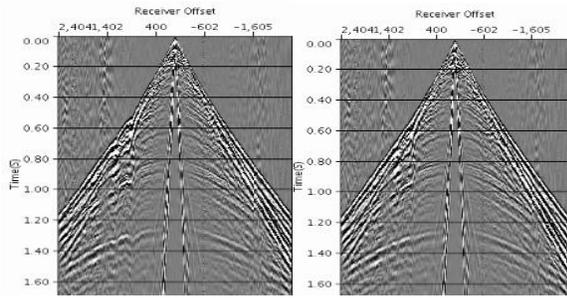
Figure 7: A 2D shot gather before (left) and after (right) the application of residual statics correction.
