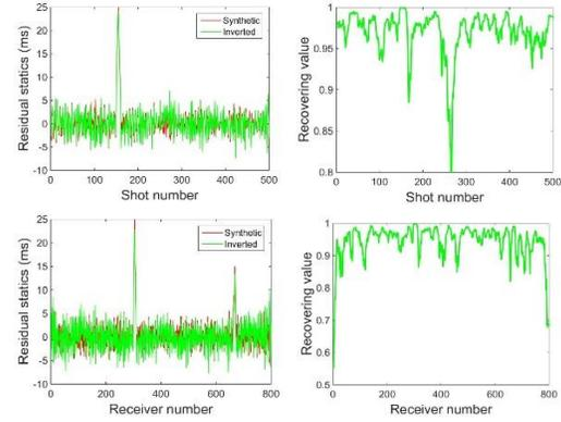
Figure 5: Recovered residual statics and resolvability with noise. The left panel is the comparison between true synthetic statics and inverted statics. The right panel is the calculated recovering degree for residual statics inversion.
