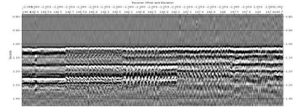
Figure 9: Common offset gather before (upper) and after (under) the application of residual statics.
