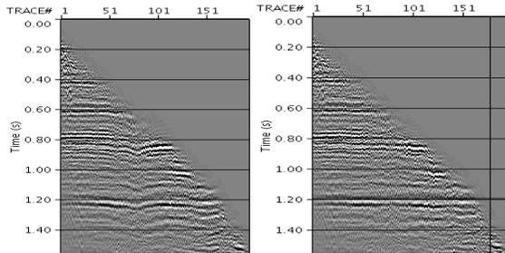
Figure 8: NMO corrected CMP gathers before (left) and after (right) the application of residual statics correction.
