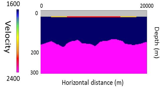
Figure 2: Undulating refractor model
