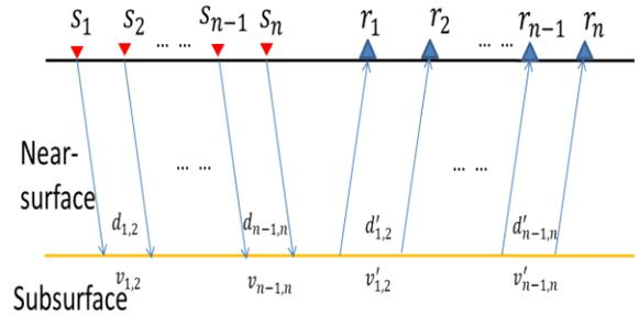
Figure 1: Schematic illustration of refraction raypath in a common offset gather.  $s_n$  and  $r_n$  represent the  $n_{th}$  shot and the  $n_{th}$  receiver, respectively.  $r_n$  detects the signal from  $s_n$ . Shot-receiver offset for each trace is same. Items with  $d$  and items with  $v$  represent the distance and the velocity, respectively, for corresponding refractor cells.
