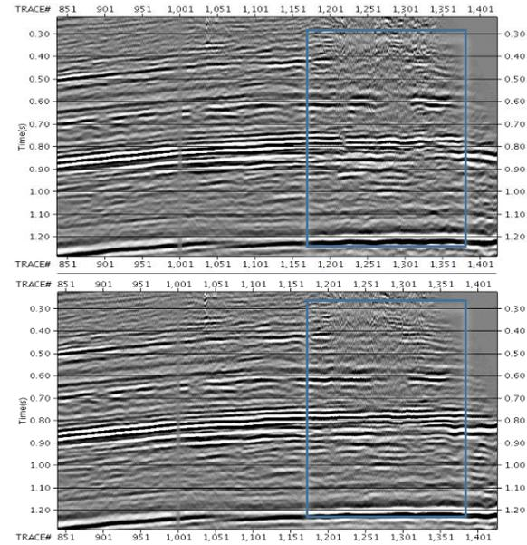
Figure 10: 2D stacked section before (upper) and after (under) the application of residual statics.
