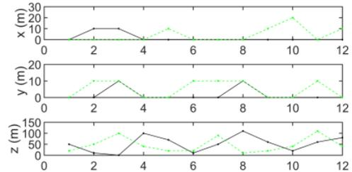
Figure 6: The calculated errors in x, y, and z direction. The black solid line represents the RMS velocity and the green dashed line represents the 1D layered velocity model.
