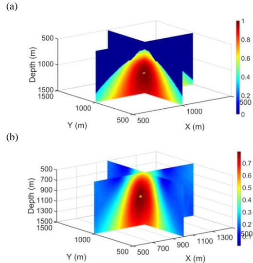
Figure 3: The stacking energy distribution of single event. (a) The result based on a 1D layered velocity model; (b) The result based on RMS velocity. The yellow star denotes the point with maximum stacking energy.
