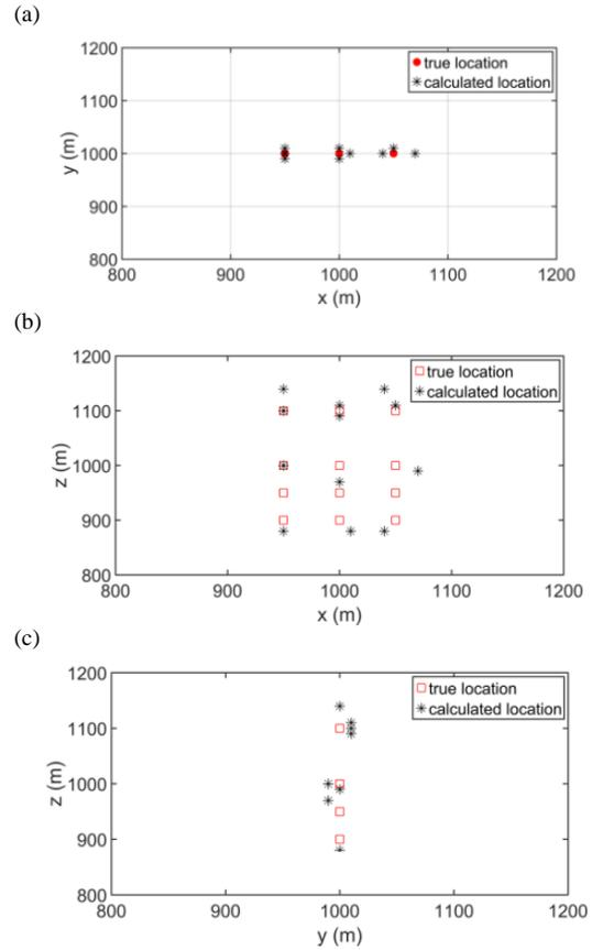
Figure 5: The calculated locations of 12 events with 1D layered velocity compared with the true locations in 2D planes. (a), (b), (c) showing the locations of 12 events in x-y, x-z, and y-z plane respectively.
