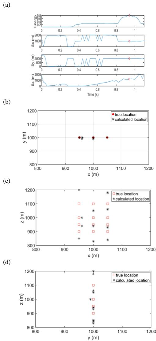
Figure 4: The RMS velocity results compared with the true location. (a) showing the energy for each parameter  $t_0$  and the corresponding location with maximum energy (red circles). (b), (c), (d) showing the calculated locations of 12 events with RMS velocity compared with the true locations in x-y, x-z, and y-z plane respectively.
