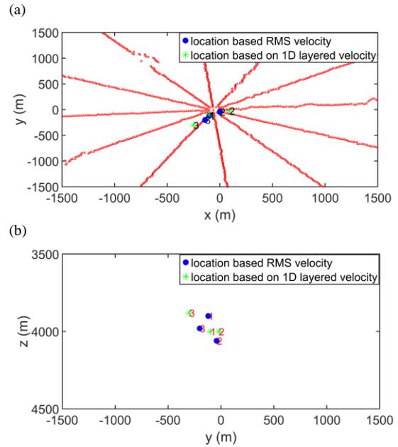
Figure 8: The location results of 3 events based on 1D layered velocity and RMS velocity in 2D planes. The same number means the same single event is located by two methods. (a) showing the locations in x-y plane with two methods. The red stars shows the receiver geometries for the microseismic events generated by hydraulic fracturing. (b) showing the locations in y-z plane with two methods.
