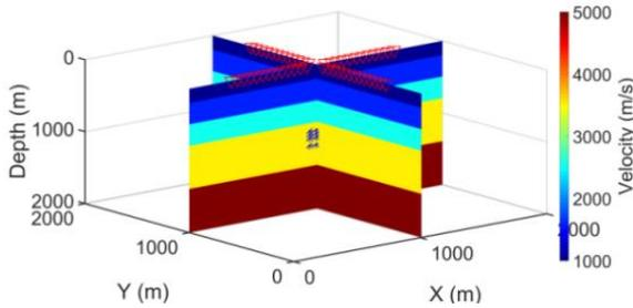
Figure 1: The velocity model and geometry of the test includes 50 receivers (red triangle) with an interval 50 m deployed along the cross line, and 12 events are represented by blue stars.
