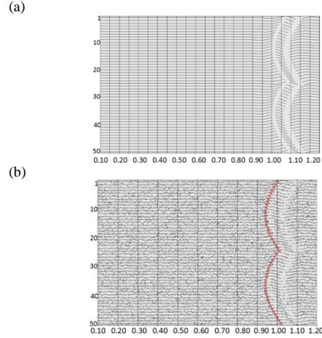
Figure 2: (a) A synthetic waveform generated for the event location (1050.0, 1000.0, 1100.0) m. (b) Above synthetics contaminated with Gaussian noises (SNR: 40%).
