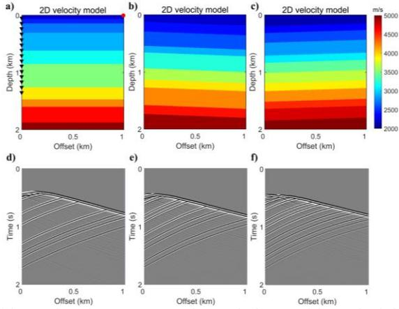
Figure 2: Three representative velocity models and their corresponding seismic images. The red dot denotes the source position and the black triangles indicate every 10th receiver (a total of 150 receivers).
