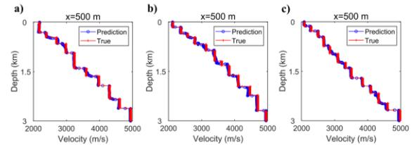
Figure 5: Vertical velocity profiles for the three test samples in Figure 4. The predicted and ground truth velocities in the velocity versus depth profiles at 500 m offset are presented.
