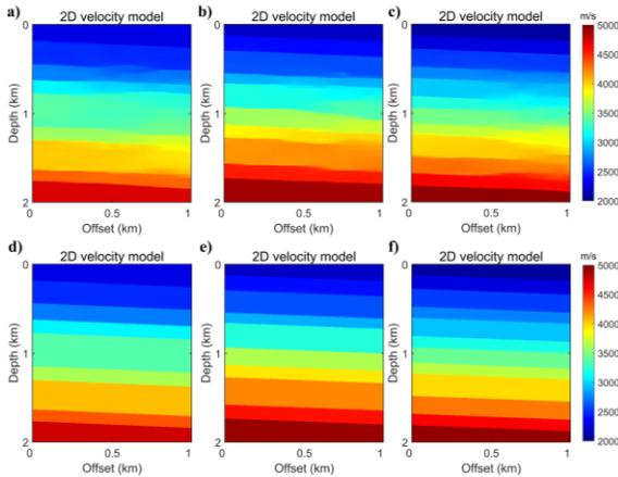
Figure 7: Comparison between the prediction of our method (a-c) and the ground truth (d-f) for the inclined layered velocity models.
