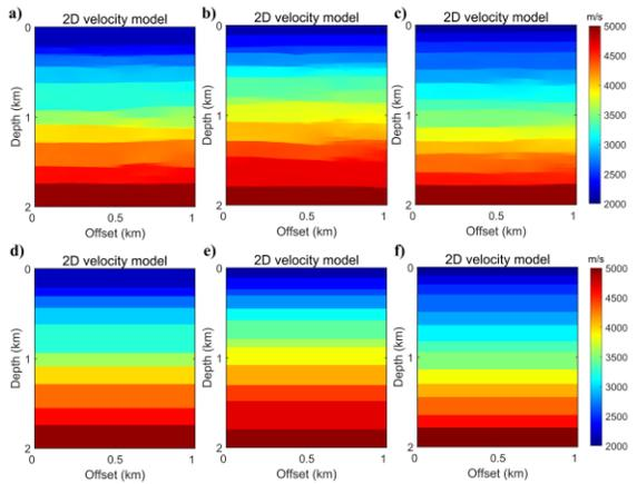
Figure 4: Comparison between the prediction of our method (a-c) and the ground truth (d-f) for the horizontal layered velocity models.
