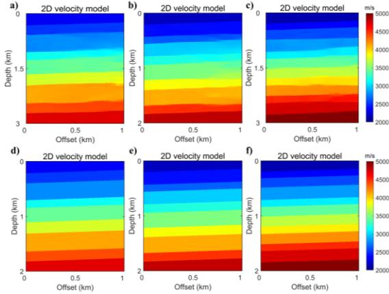
Figure 6: Comparison between the prediction of our method (a-c) and the ground truth (d-f) for the inclined layered velocity models.
