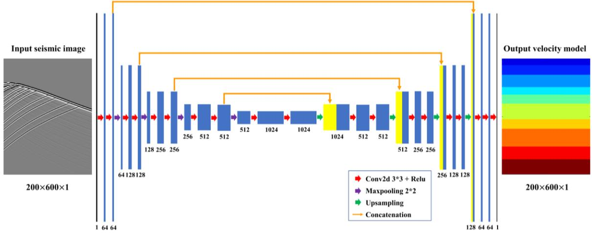
Figure 1: A modified convolutional neural network (U-Net) for 2D velocity model building.
