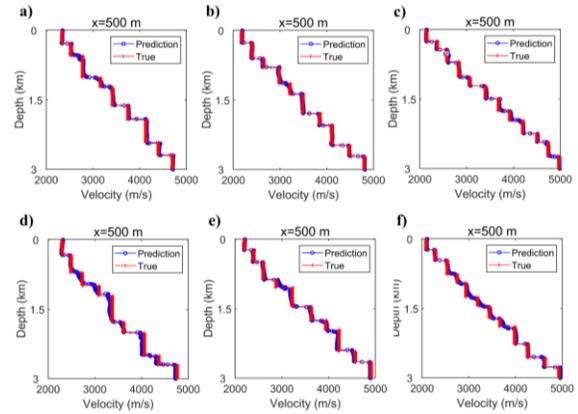
Figure 8: Vertical velocity profiles for the six test samples in Figures 6 (a-c) and 7 (d-f). The prediction and ground truth velocities in the velocity versus depth profiles at 500 m offset are presented.
