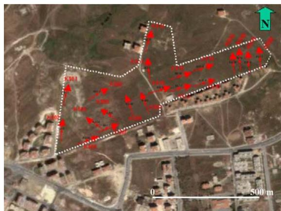
Figure 1. Location map for the seismic survey conducted within the residential development project site. The survey consists of refraction profiling at 20 locations.
