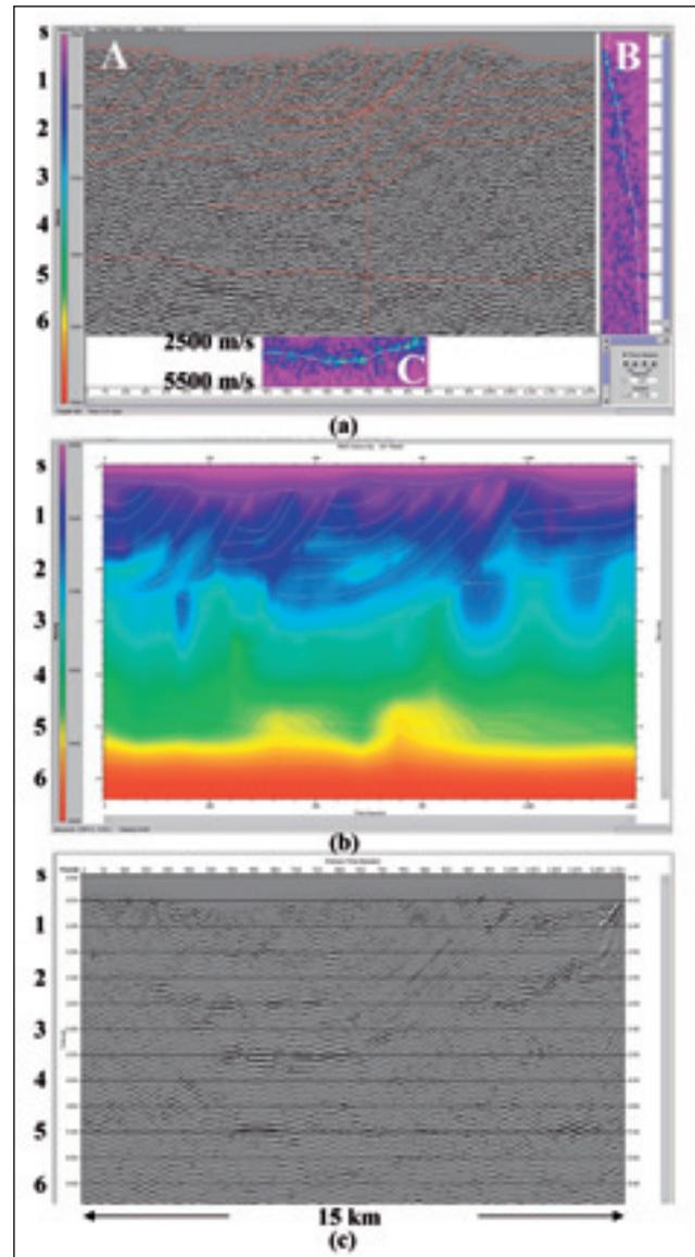
**Figure 3** (a) Three cross-sections of a velocity cube in time --- A: image panel for a specific velocity, B: semblance spectrum at a specific location along the line traverse, and C: time slice or horizon-consistent semblance spectrum; (b) the RMS velocity strands and the RMS velocity field derived from the velocity cube in (a); and (c) image from prestack time migration using the RMS velocity field in (b).
