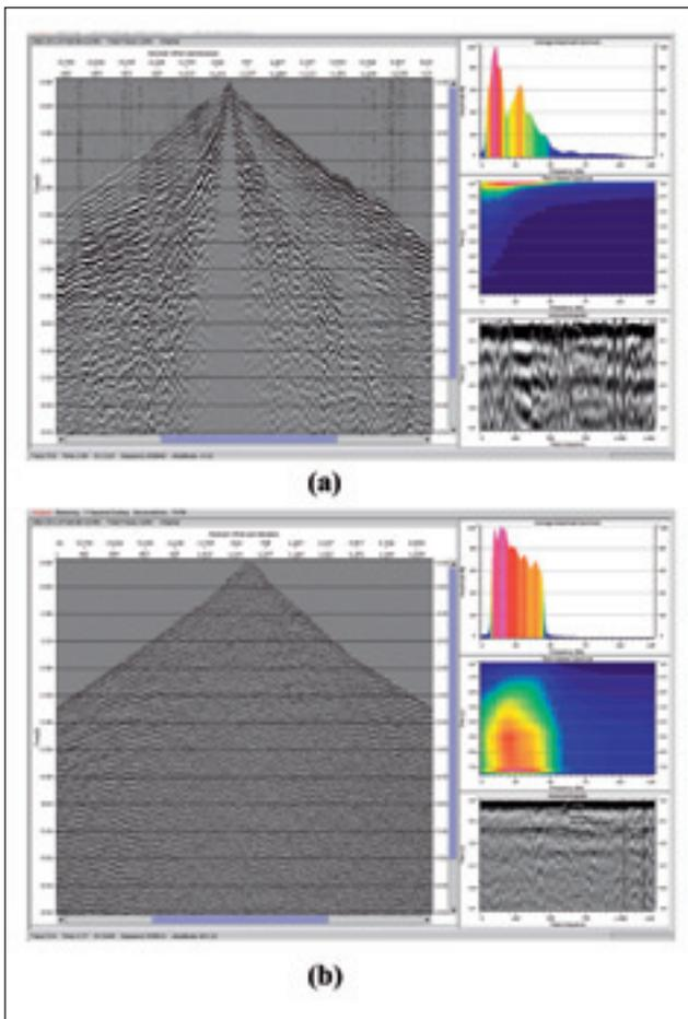
**Figure 2** (a) A shot gather with its average amplitude spectrum (top right), time-variant spectrum (center-right), and autocorrelogram (bottom-right); and (b) the same shot gather after  $t$ -squared scaling, deconvolution, time-variant spectral whitening, statics corrections, and  $f$ - $x$  prediction filtering to remove the residual coherent linear noise associated with ground-roll energy.
