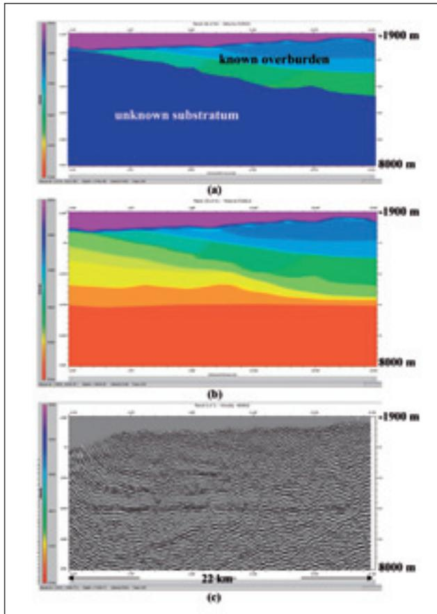
**Figure 4** (a) A velocity-depth model at an intermediate stage of model building based on layer-by-layer estimation of layer velocities and delineation of reflector geometries; (b) final velocity-depth model; and (c) image from prestack depth migration using the velocity-depth model in (b).
